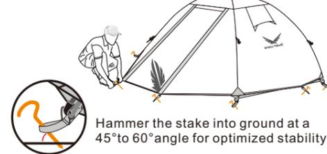
**Step 6** Guy lines are attached to the fly for additional stability. Extend the guy lines and place loop over stake. Stake to the ground and adjust the slider to make guy lines tight.
