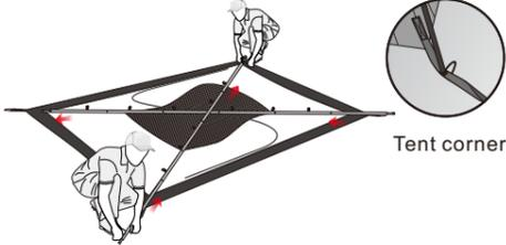
**Step 3** Flex the poles into an upward position to raise the tent. Clip the hook at the center of the top roof to the intersection of two poles and clip the rest hooks to the poles.
